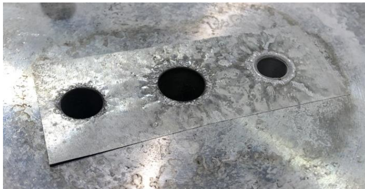
Figure 18. Shim After an Experimental Run
