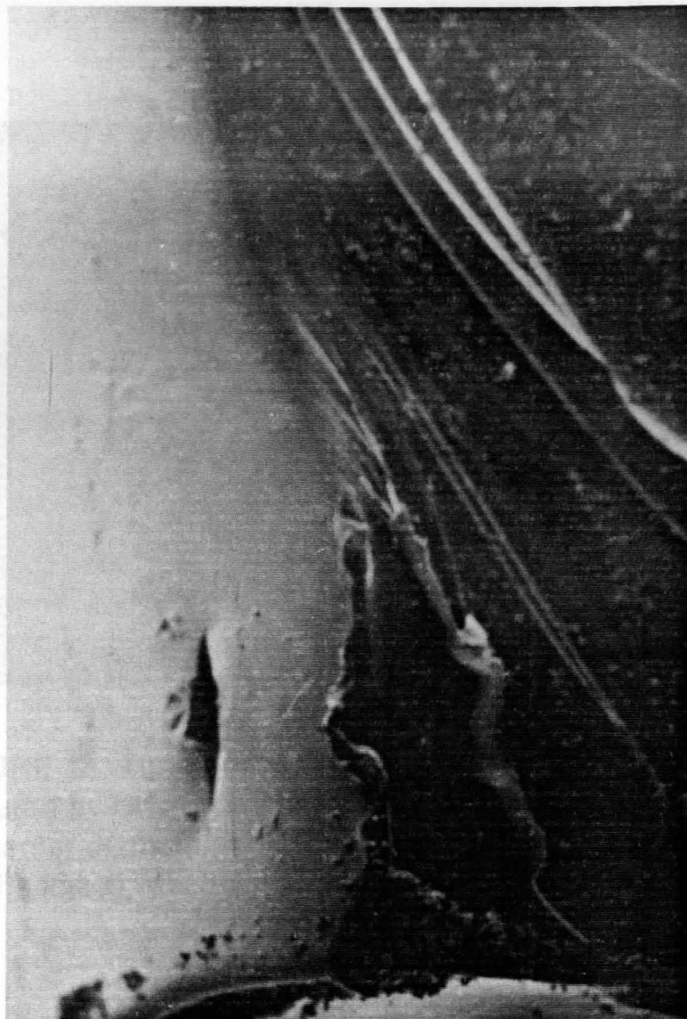
FIGURE 17. (M = 45) SEM photograph of bending fracture surface. Features to be noted are voids, tear fracture, crazing, white spheres, and fracture bands.
