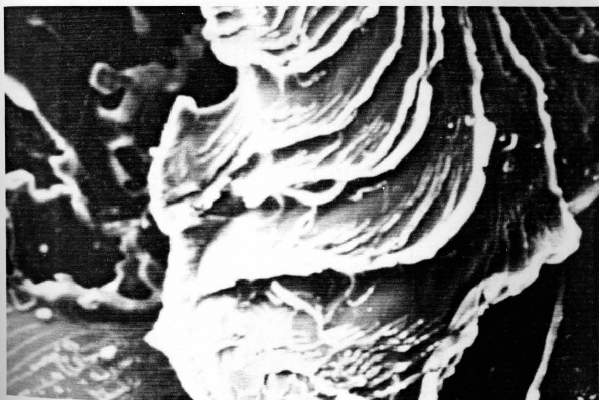
FIGURE 21. (M = 142 top, M = 380 bottom) SEM photographs of fracture surface of Charpy impact test showing swirling concave areas and enlargement of these features.
