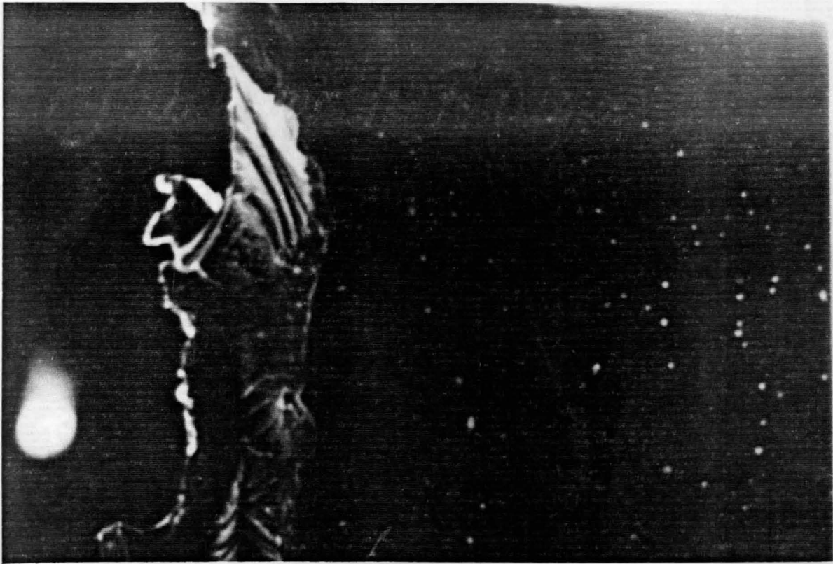
FIGURE 29. (M = 46) SEM photograph of the tear fracture that was caused by cutting the sample.
