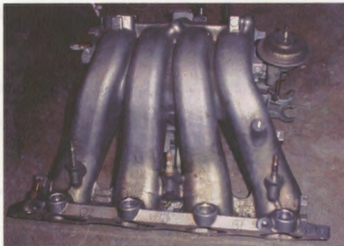
Figure 4.1: Stock Variable Geometry Acura Integra GSR Intake Manifold
