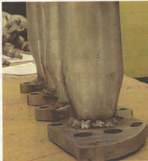
Figure 4.12: Runner Taper Welded to Head Flange
