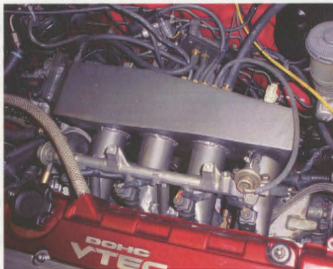
Figure 4.2: Optimized Intake Manifold on the Car
