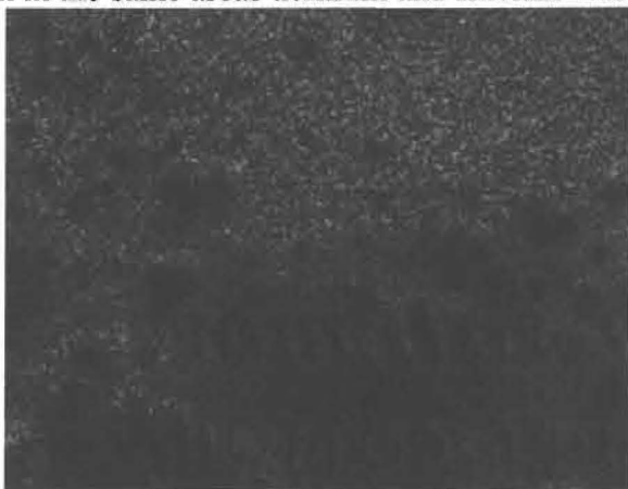
Fig. 5.7 X-ray Map of nitrogen (brown). The lighter regions indicate the presence of nitrogen in the same areas titanium and fluorine were found.
