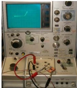
Figure 53: Tektronix 576 I-V curve tracer attached to the custom diode test rig.
