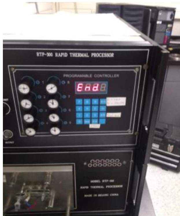
Figure 22: A temperature-controlled furnace, (MODEL RTP-300 RAPID THERMAL PROCESSOR).
