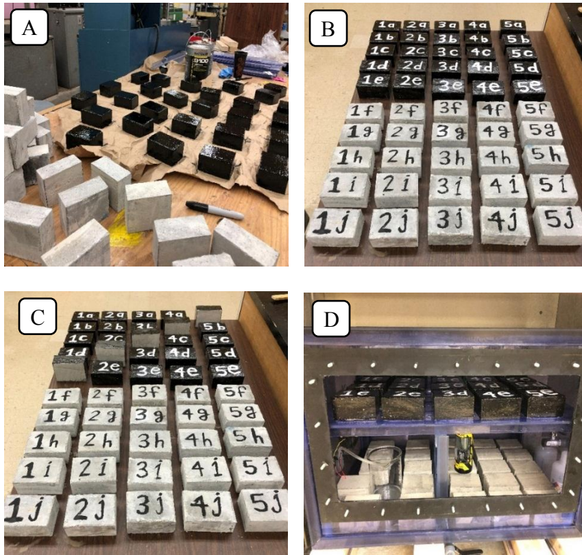
Figure 3-7, Epoxy coating and numbering of coupons (pictures by Mostafa Nasr)
