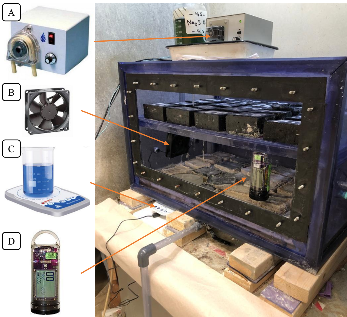
Figure 3-10, H_2S gas generation process and tools, (A)peristaltic pump, (B)waterproof axial fan, (C)magnetic stir plate, (D) AcruLog TM H_2S gas data-logger.
