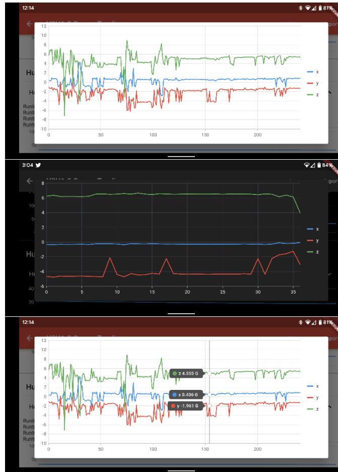
Figure 4-5 Screenshots from the YSU Bluetooth Suite application showing full screen plot viewing. From top to bottom: Plot viewing (light mode), plot viewing (dark mode), point selection (light mode).
