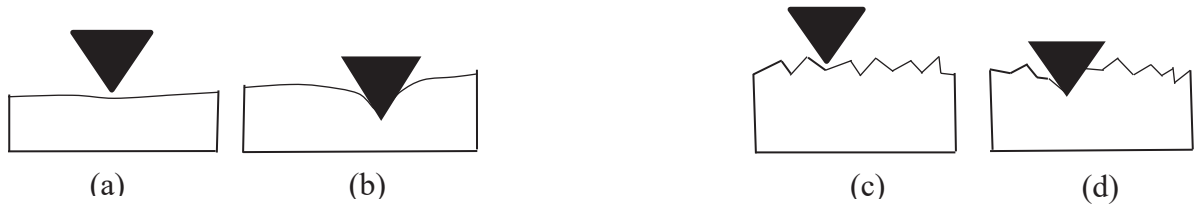
Figure 3-19 Indentation test on different types of surfaces: (a) before indentation on a flat surface, (b) after indentation on flat surface, (c) indentation on the twinned surface, (d) after indentation on the twinned surface
