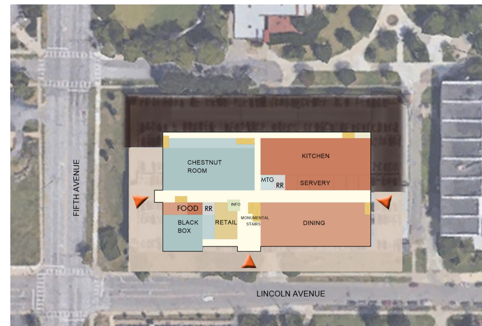
The crossroads created by the north-south and east-west circulation in the proposed building simplifies wayfinding throughout the building and strategically sorts the major space functions on each floor.
