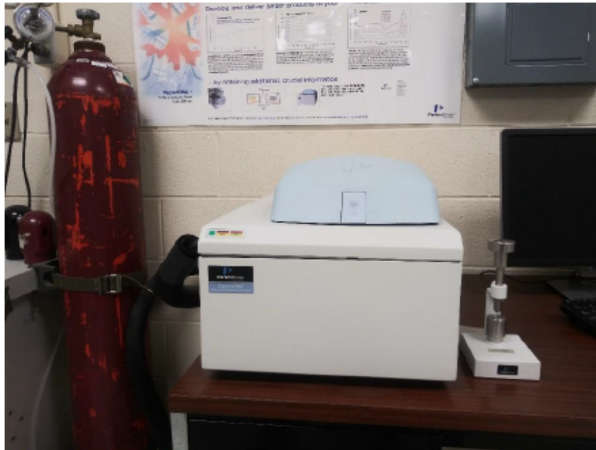
Figure 2.6 Perker-Elmer Diamond DSC for investigating phase transformation.
