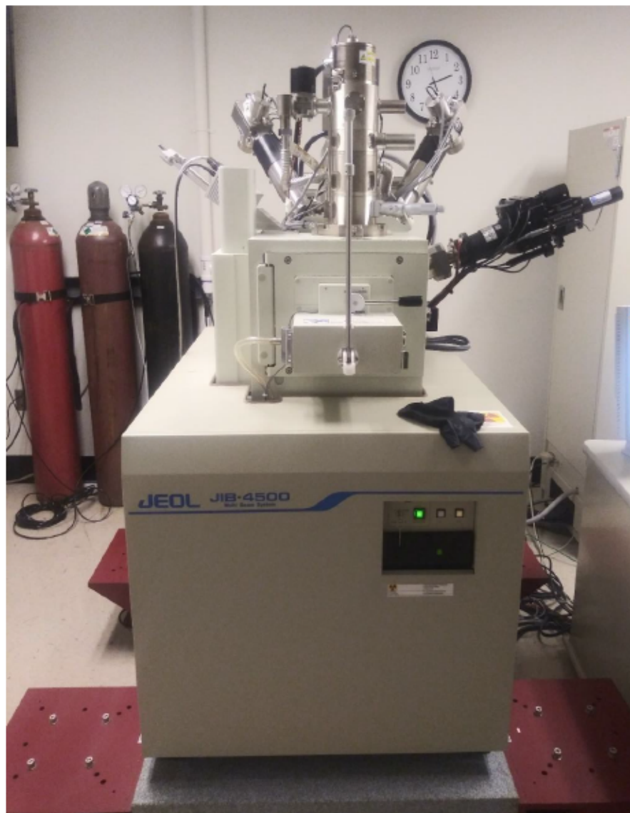
Figure 2.4 JEOL JIB 4500 Multi Beam System SEM/FIB equipped with EDAX Apollo XV detector for chemical analysis.
