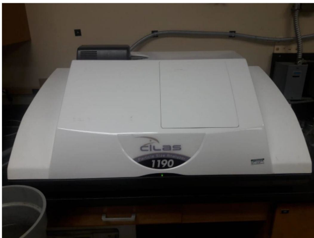
Figure 2.3 Cilas 1190 particle size analyzer used in this research.
