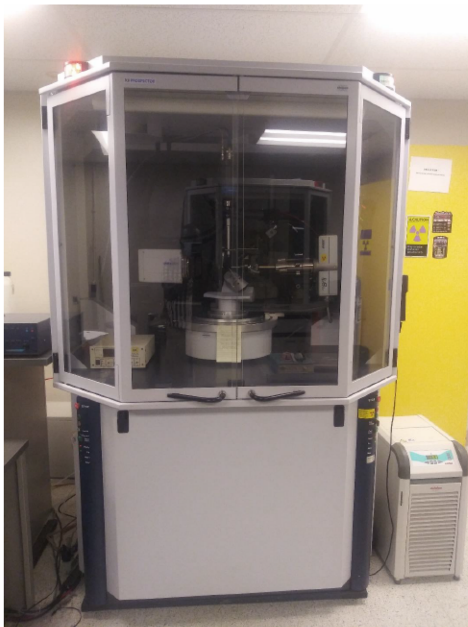
Figure 2.5 Bruker AXS X8 Prospector single crystal diffractometer for structural analysis and phase identification.
