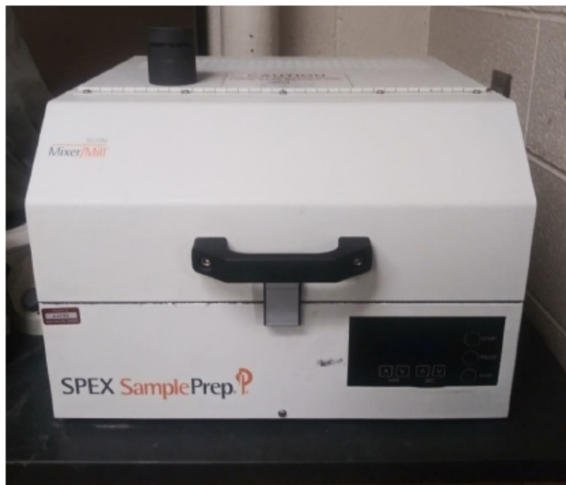
Figure 2.1 SPEX 8000M ball milling machine used in preparing Ni-Mn-Ga powders.
