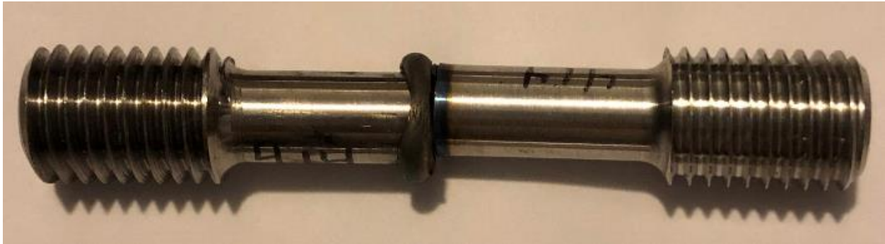
Figure 3-16. Specimen with wrapping deformation along the weld interface.
