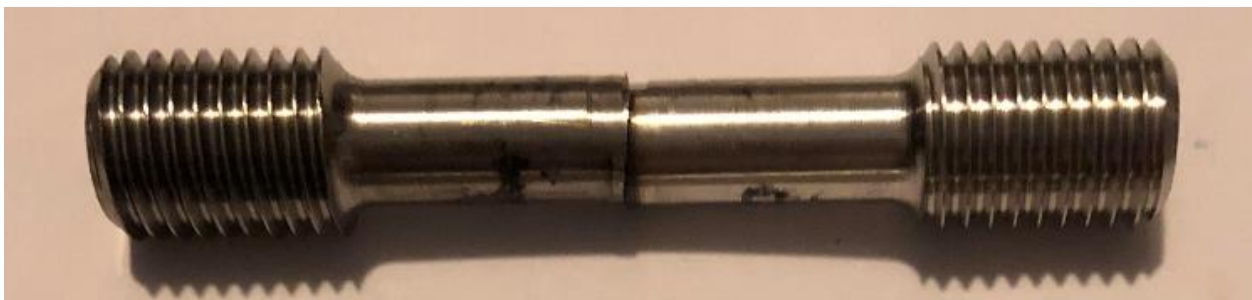
Figure 3-15. Specimen with plastic buckling.
