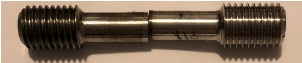
Figure 3-17. An example of a specimen that did not achieve successful bonding.
