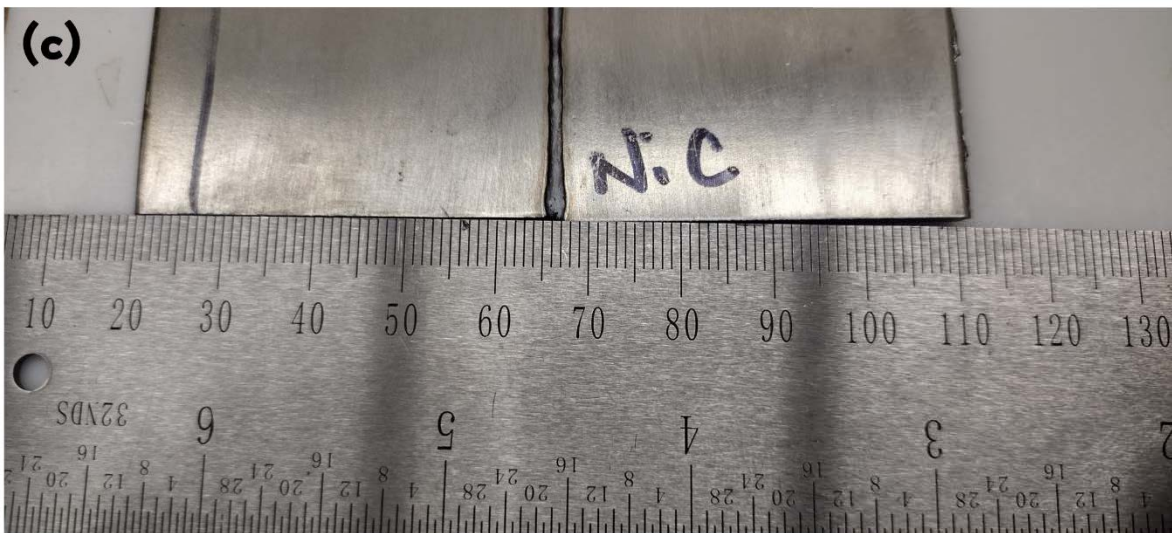
Figure 5-6. Trial 2 LW results for velocities (a) 5 mm/s, (b) 20 mm/s, and (c) 100 mm/s.
