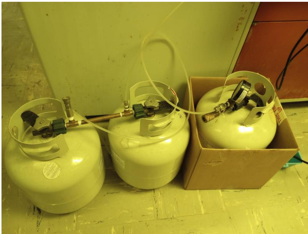
Figure 3.30: Pressurized gas cylinders containing landfill gas.
