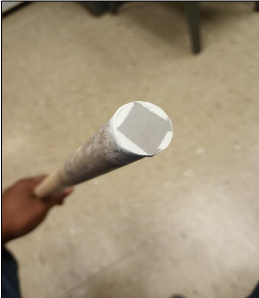
Figure 2.10: The coated YSZ button cell with platinum on both sides and testing for its conductivity using the multimeter
