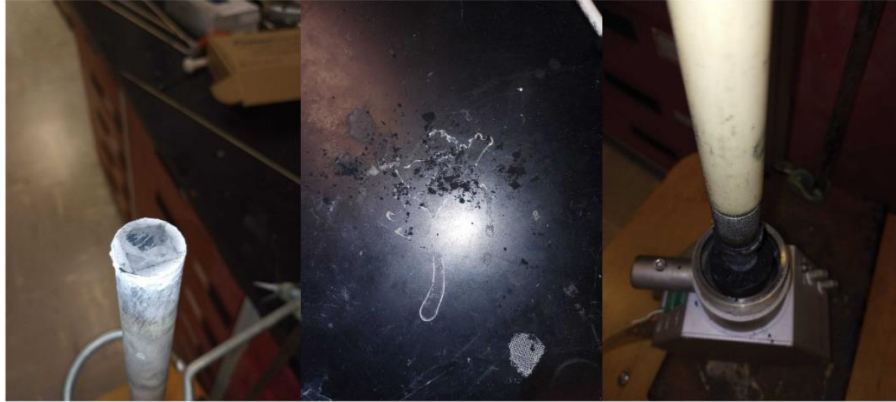
Figure 3.13: Carbon soot tainting the Pt button cell and the Probostat.
