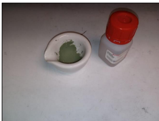
Figure 2.12: Ni cermet formulation diluted with \alpha -terpineol.
