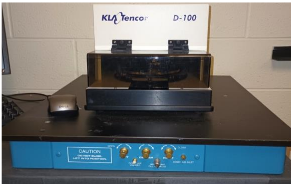
Figure 13. KLA Tencor D-100 stylus profilometer in YSU laboratory.
