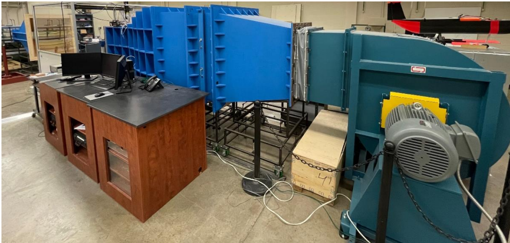
Figure 3-18: Open test section wind tunnel at YSU.
