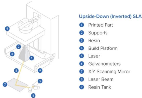
Figure 3-1: Schematic diagram of SLA printer [22].
