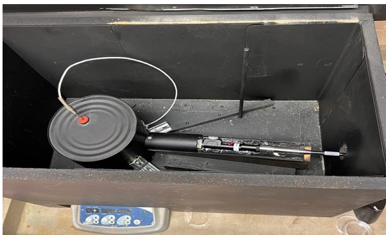
Figure 6: Raman probe fitted in dark box.
