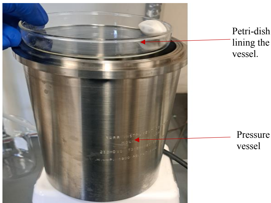
Figure 46. The One-liter Parr Non-stirred Reactor Pressure Vessel
