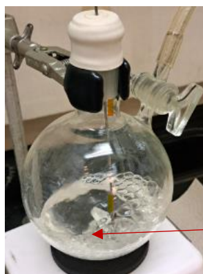
Figure 21. Filtered Carbene Ready for Carboxylation
