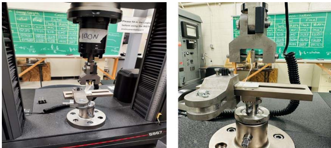
Figure 4.5. Setup of Adhesion Apparatus.
