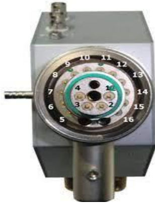
Fig 2.4: Position of pins on Probostat™
