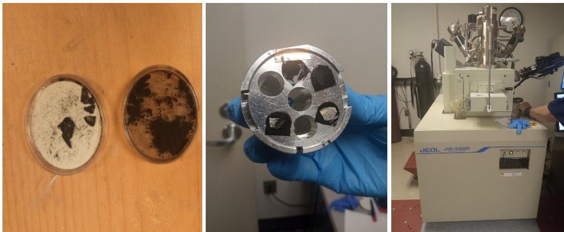
Fig 3.25: Post-analysis of black deposits and Ni/YSZ/LSM
