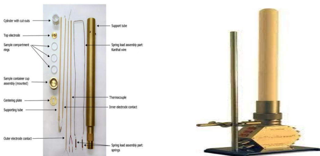
Fig 2.3: Diagram of Probostat™
