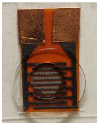
Figure 6.1. Picture of the IDE touch pad design with a polycarbonate backplate and a PDMS spacer.
