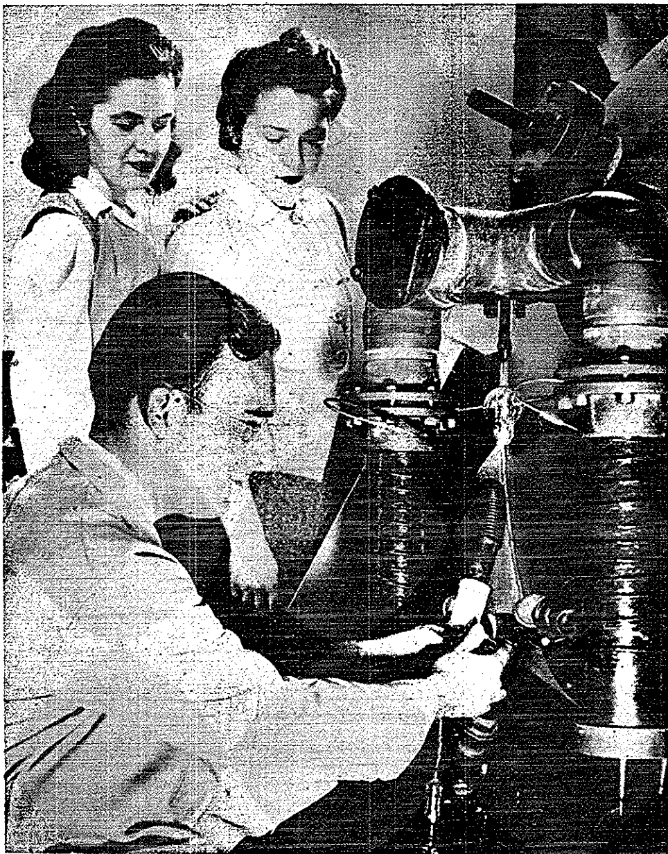
Midget Atom Smasher — Dr. W. R. Kanne, research physicist at Illinois Tech, Chicago, explains the "target end" of what will probably be the world's smallest atom smasher to two of Tech's co-eds. The tiny electrostatic generator will be ready for use soon.
