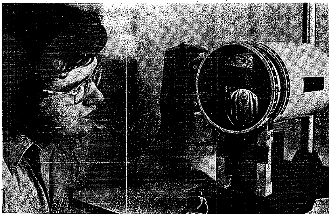
PHOTO-ELASTICITY — Michael Birchak, president of the YSU chapter of the American Society of Mechanical Engineers, views a demonstration model of photo-elasticity, in which polarized light shows stress concentrations in a piece of plastic. This is only one of the Dean's Council-sponsored display of engineering exhibits in the Engineering Science Lobby being shown through today.
