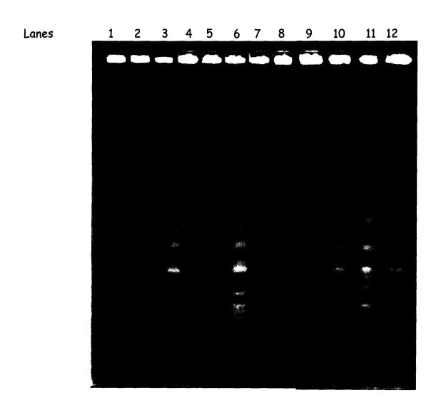
Fig. 16: PFGE results of 2000 and 2001 harvest season yeast *Pichia* and *Hanseniaspora*. A 1% Pulse Field gel subjected to 24 hrs. at 6 v/cm with an initial switch time of 60 seconds and a final switch time of 120 seconds with an angle of 120°.
