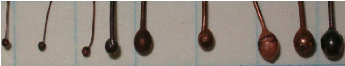
Figure 27: Several dimensions of spherical contacts in various stages of construction.
