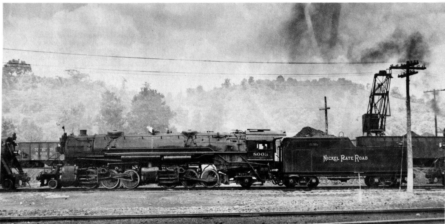
WEARING NICKEL PLATE LETTERING but retaining her W&LE number, 2-6-6-2 8003 shows off her classic USRA figure in this 1950 broadside in the Pine Valley engine terminal. In January 1951 she became NKP 942 and continued to work coal trains out of Pine Valley until March 21, 1953.
