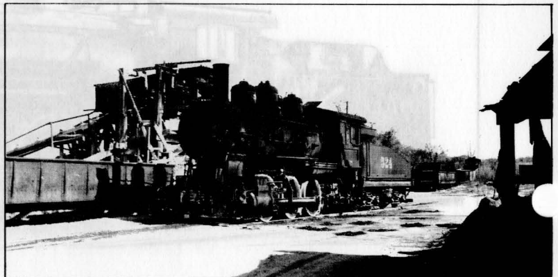
Northern Indiana Gravel Co. #524, 0-6-0, ex-Wabash #524, B-6. In rear distance beyond end of cars is the mogul A.I.Co. #8. Oct. 1949. All rights reserved.
