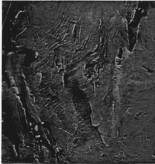
Figure 19. Crack Pattern Found on Cylindrical Surface of Jewett Hip Nail-Plate (SEM), at 400X.
