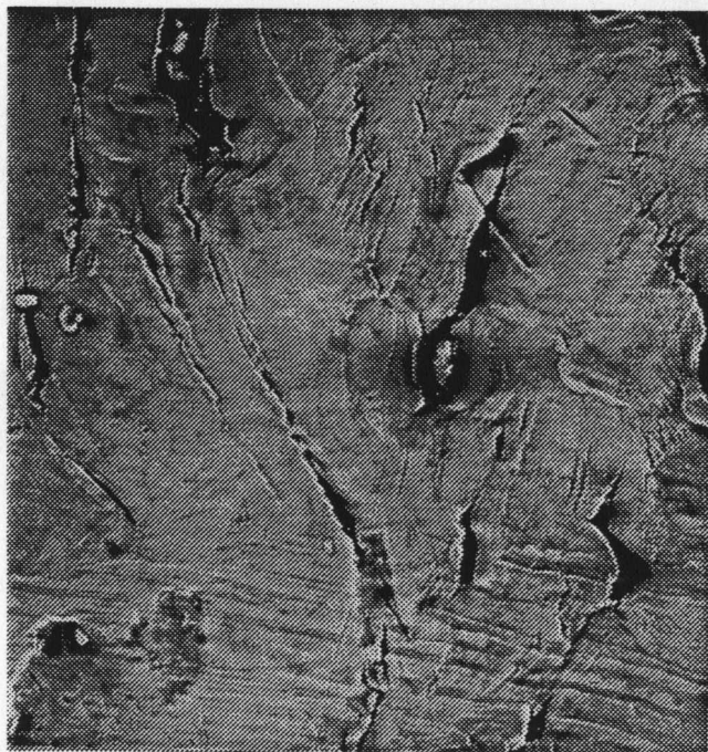
Figure 20. Crack Pattern Found on Cylindrical Surface of Jewett Hip Nail-Plate (SEM), at 450X.
