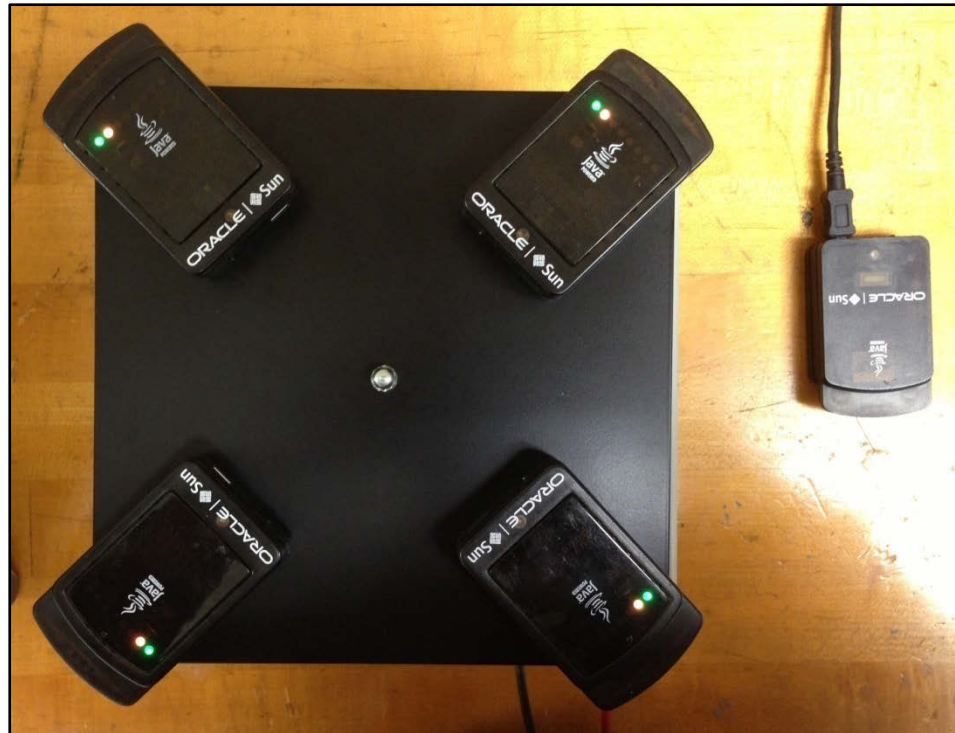
Figure 22 Setup of 4 Free-Range SPOTS on Vibration Plate
