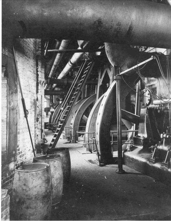
Figure 3-7: Youngstown's William Tod Co. furnished all of Andrews & Hitchcock's blowing engines from 1896 to 1910 (and possibly prior to 1896, however, no records exist). In 1910, the company utilized six vertical blowing engines to furnish the blast air for the two furnaces. The installation of two Mesta horizontal engines in 1915 resulted in the removal of several of the older vertical engines.
