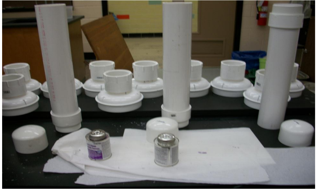
Figure 3.3: Storm Water Samplers and PVC Adhesive to Attach Lid.
