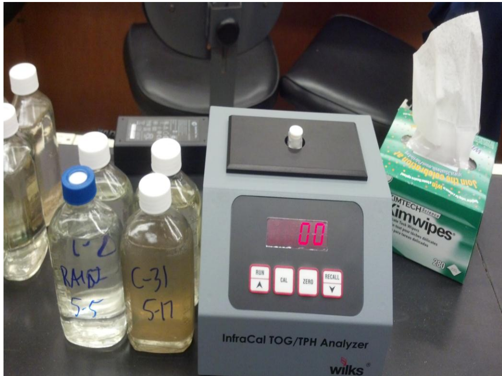
Figure 3.9: Analysis of Total Oil & Grease using Wilks InfraCal TOG/TPH Analyzer
