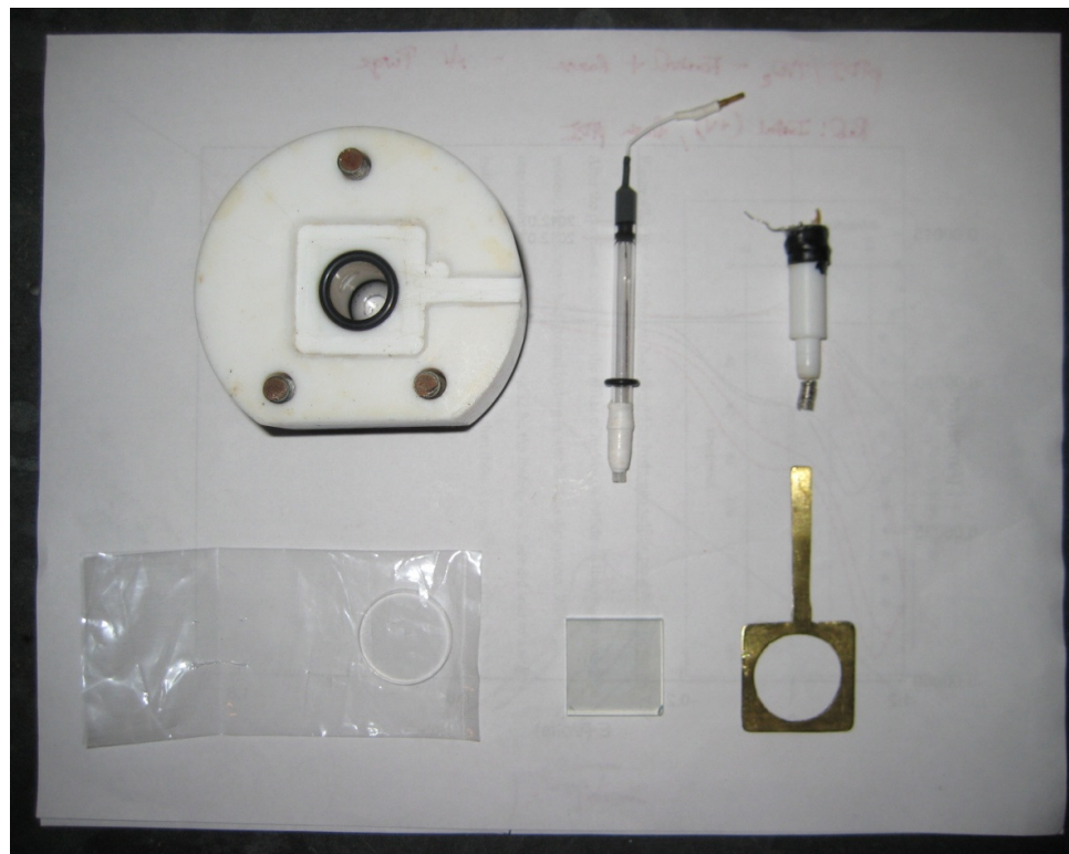
Figure 2.3.8: Cell components with side view of cell body
