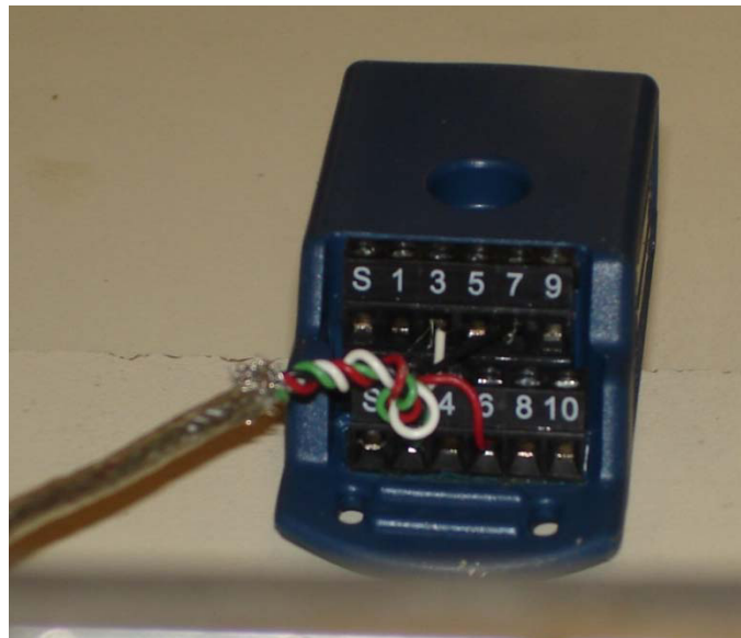
Figure 6.7 RJ50 cable with attachment terminals for load cells
