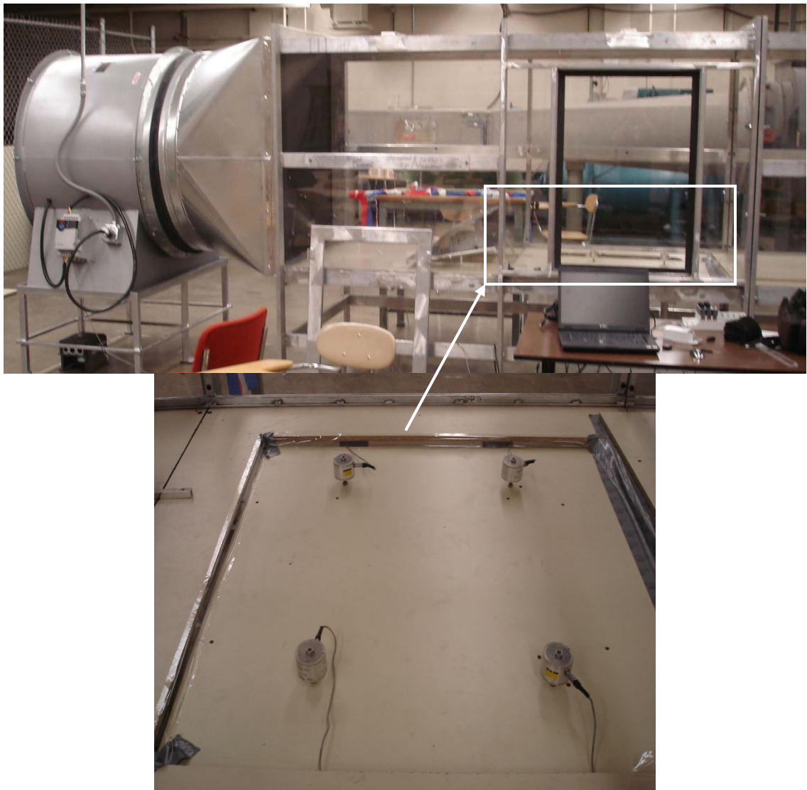
Figure 5.10 Photograph of wind tunnel instrumentation showing load cells on the testing floor for wind uplift force measurement
