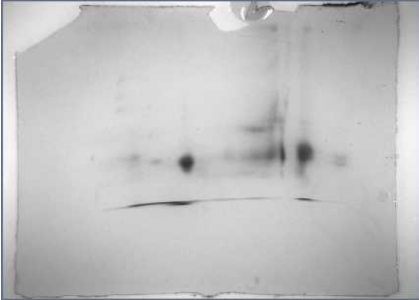
PURE RICIN reduced, 4-16-06 Comassie, 5uL Sample, 120uL RB, 10% 7cm gel, 5ug/uL Bottle (Figure 5A)
