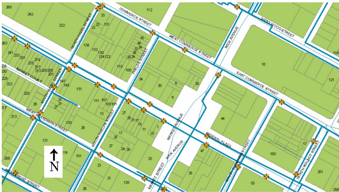
Figure 3-10. GIS for Section of Sample Area, Showing Base Map with Waterlines and Hydrants Layers.
