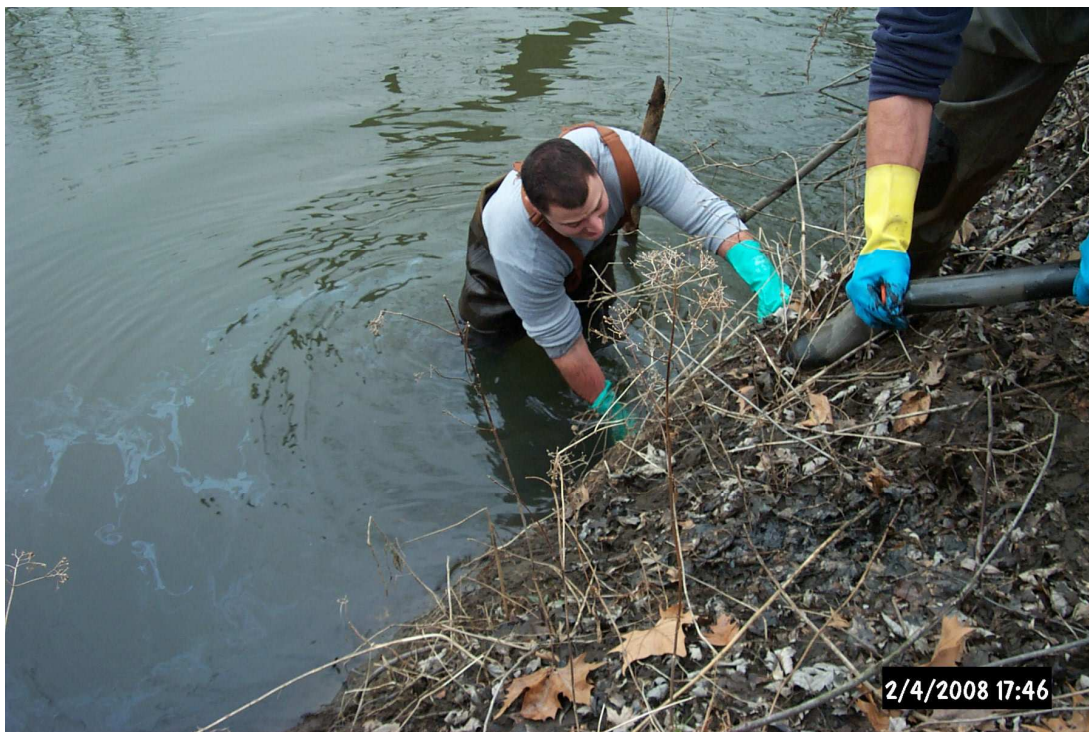
Fig. 3 – Taking a contaminated sediment core from Lowellville, Ohio river bank via the water
