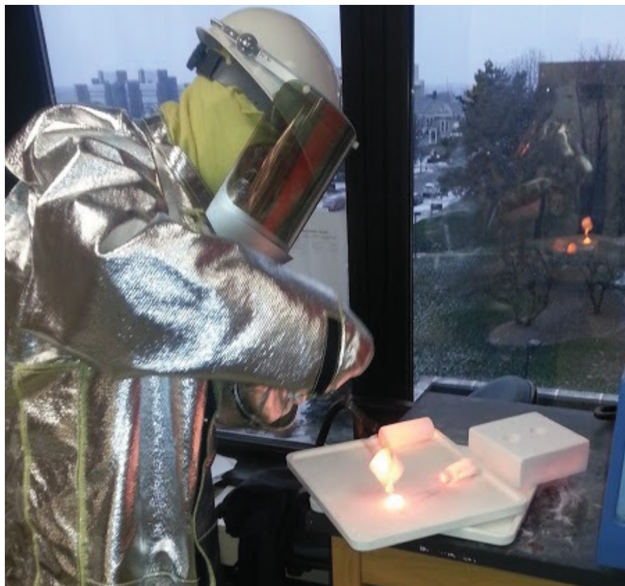
Figure 4.3 Pouring out the molten aluminum and sample pellet from crucible.
