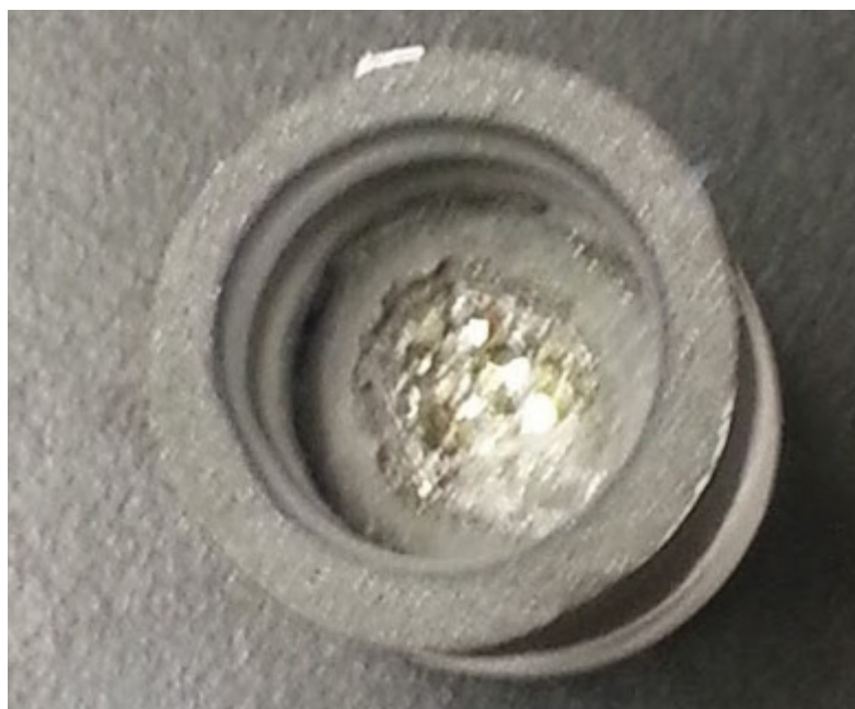
Figure 6.8 Image of crystals formed on the top of the aluminum melt
