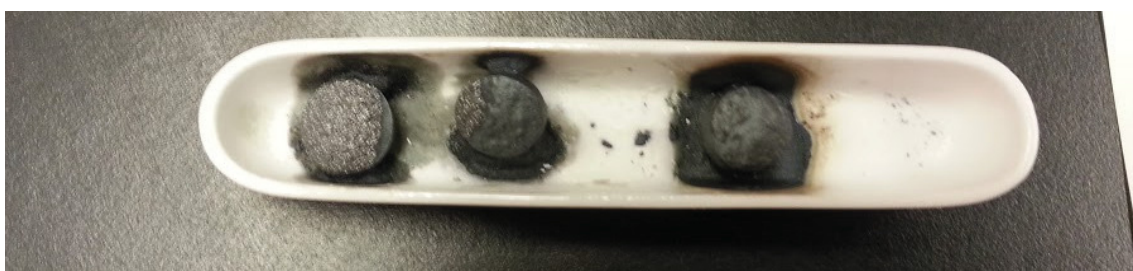
Figure 5.12. Sample of Fe 2 O 3 and AlN sintered together for 36 hours at 1450°C.
