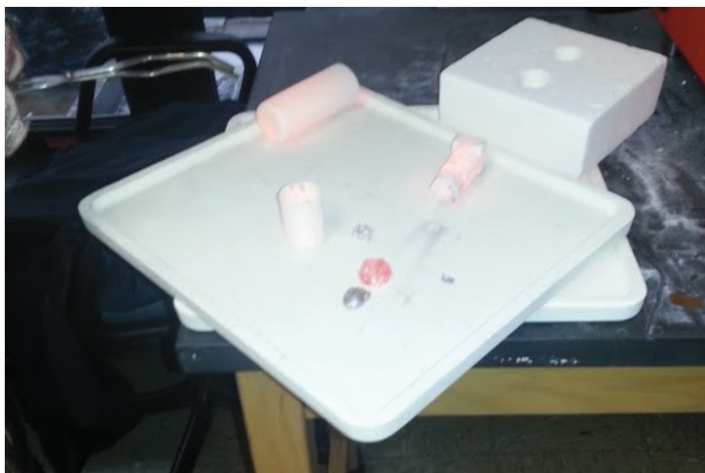
Figure 4.4 Cooling aluminum after being poured out onto tray. Sample pellet is on the middle of the tray.
