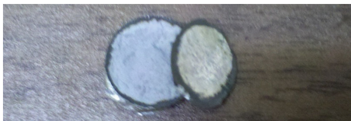
Figure 6.1. Sialon composite has fallen apart after grinding.
