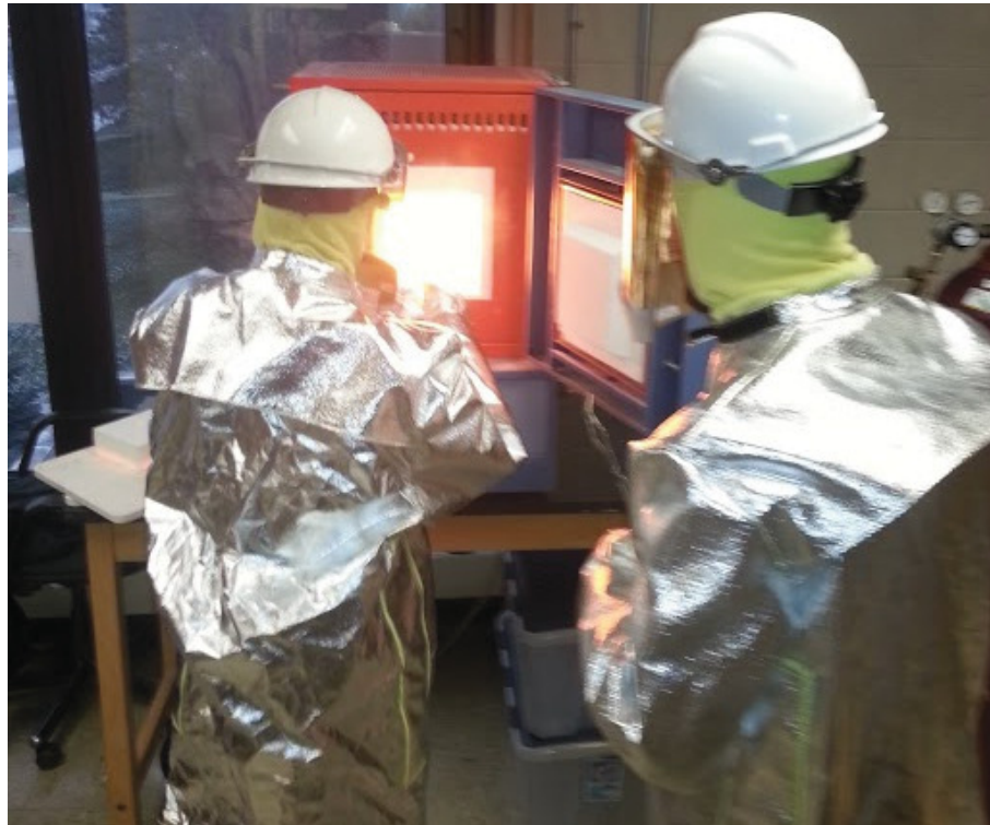
Figure 4.2 Removal of crucible and sample pellet from the box furnace
