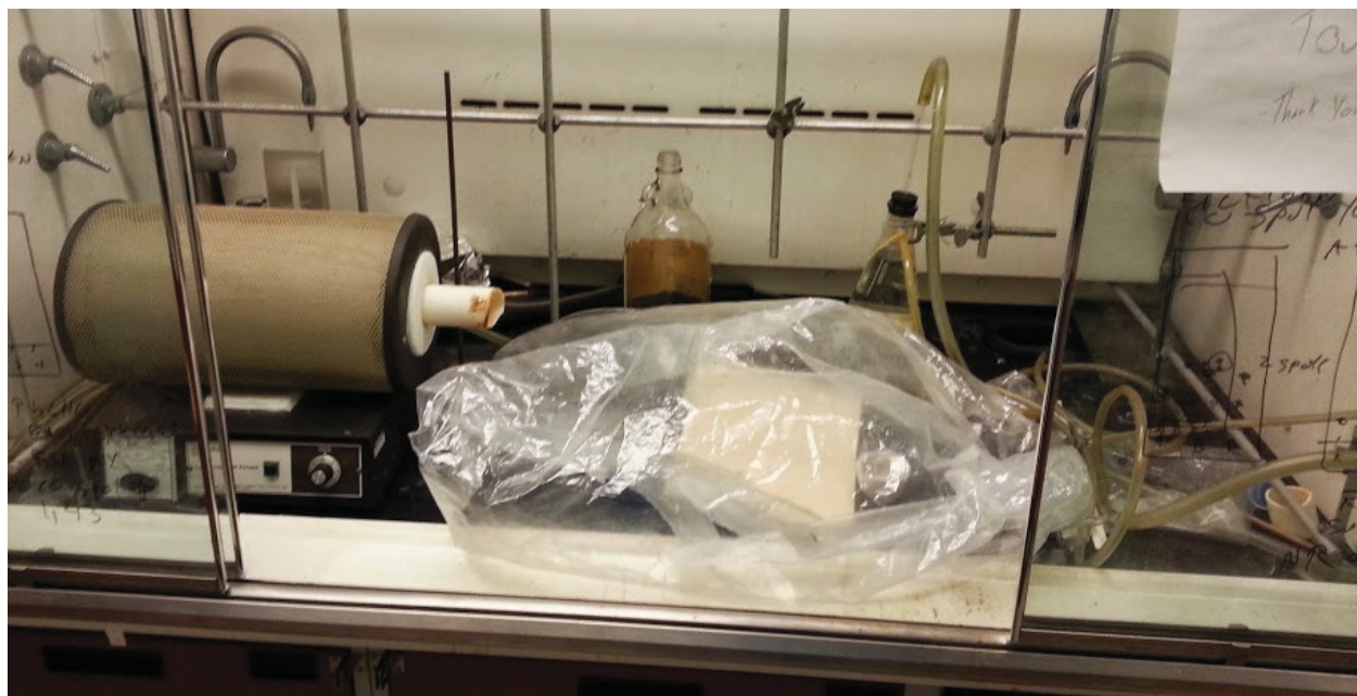
Figure 5.10 Setup used to react \text{Fe}_2\text{O}_3 with ammonia in an atmosphere without oxygen.
