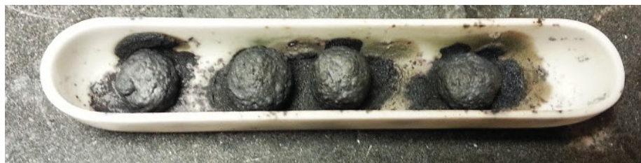
Figure 5.14. \text{Fe}_2\text{O}_3 mixed with AlN and sintered for 36 hours at 1450^\circ\text{C}
