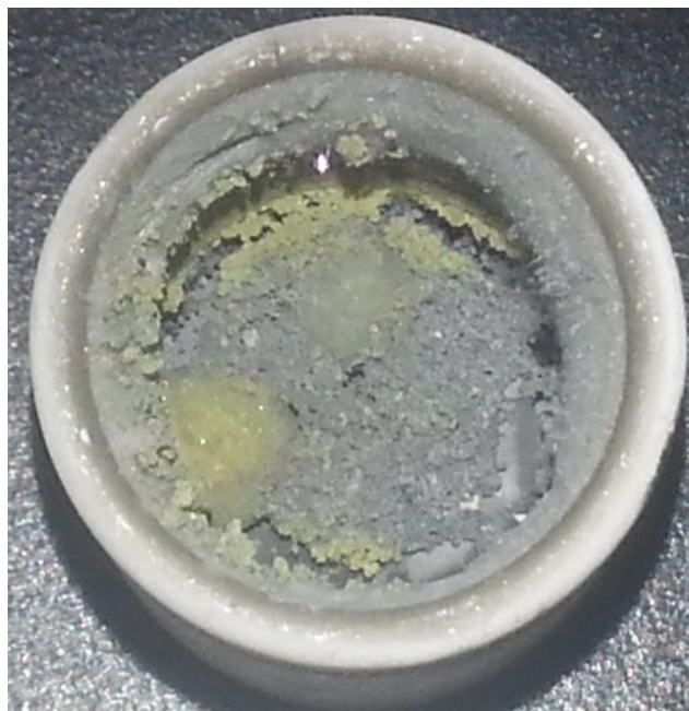
Figure 6.5 Crucible after attempted transformation via tube furnace.
