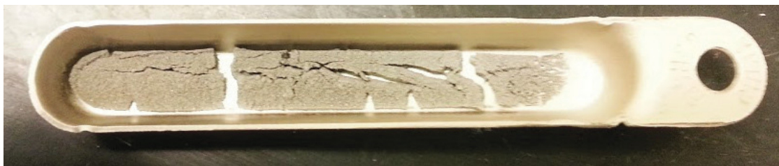
Figure 5.3. \text{Fe}_3\text{O}_4 after ammonolysis at 1000^\circ\text{C} .
