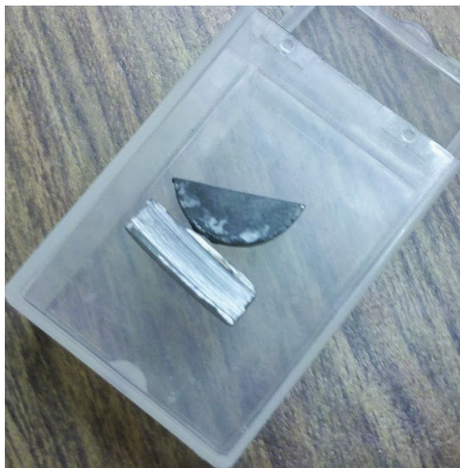
Figure 6.22 Photograph of transformed \text{SrSi}_2\text{O}_2\text{N}_2 pellet after being cut in half.
