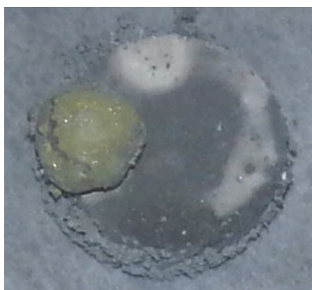
Figure 6.6 Pellet after attempted transformation via tube furnace.
