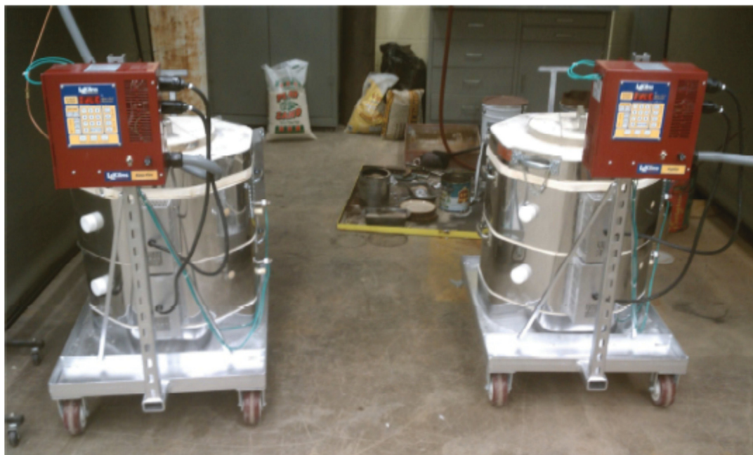
Figure 4.1 Photograph of small scale LL Kilns used for laboratory transformations.
