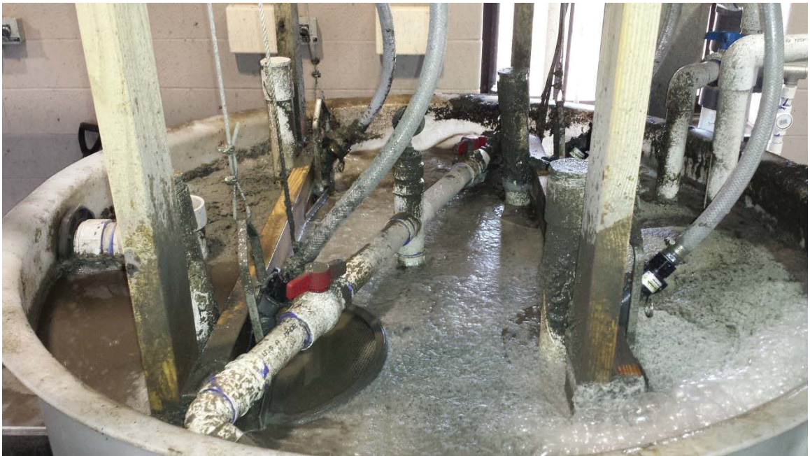
Figure C.12: Foaming in process tank 1
