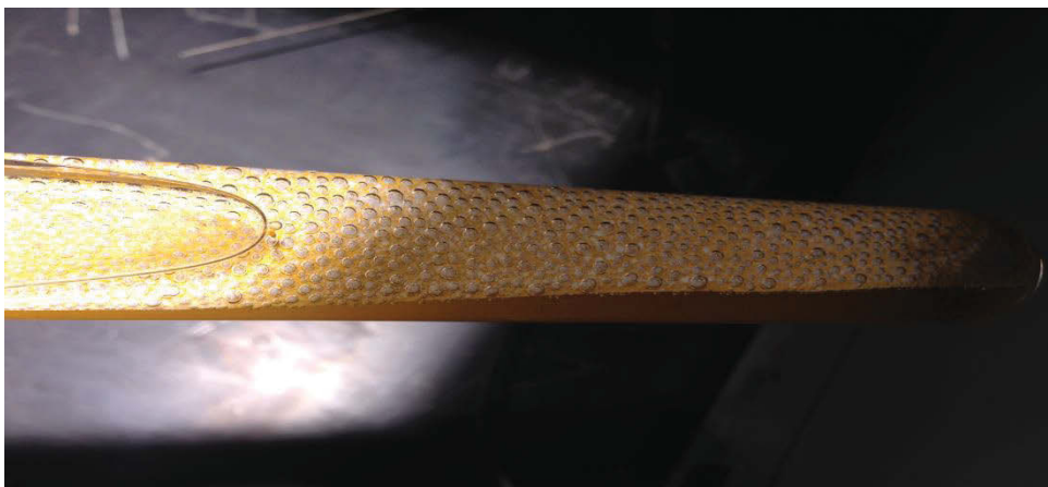
Figure 3.20. Bubbles of hydrogen gas on abraded Teflon strip
