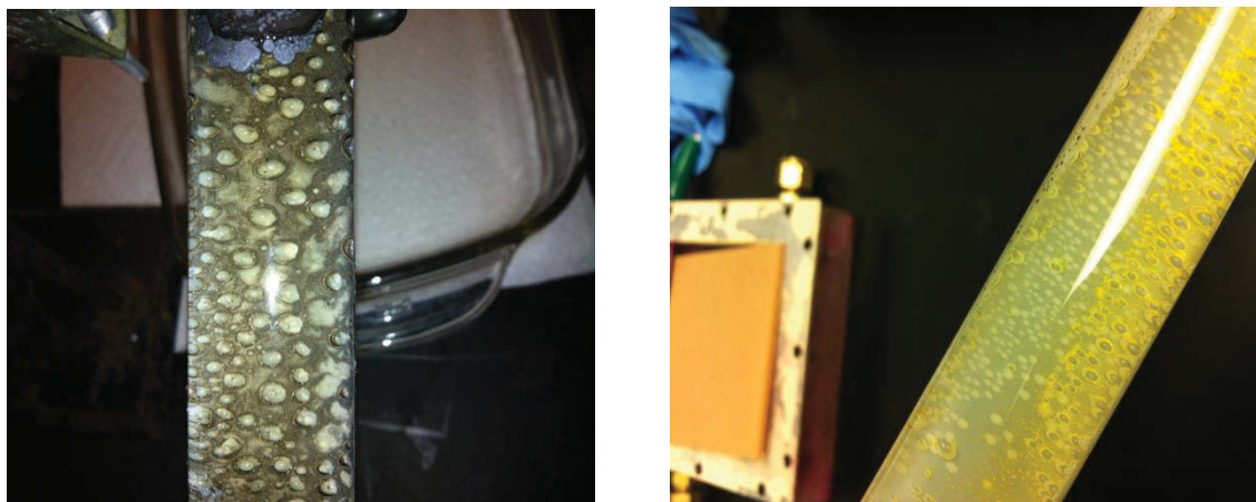
Figure 3.19. Bubbles of hydrogen gas on Teflon strip
