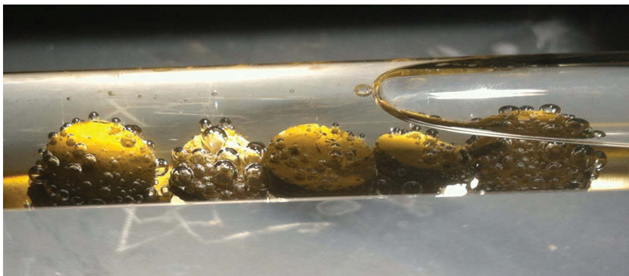
Figure 3.21. Bubbles of hydrogen gas rising from pellets made of Teflon powder and platinized CdS photocatalyst
