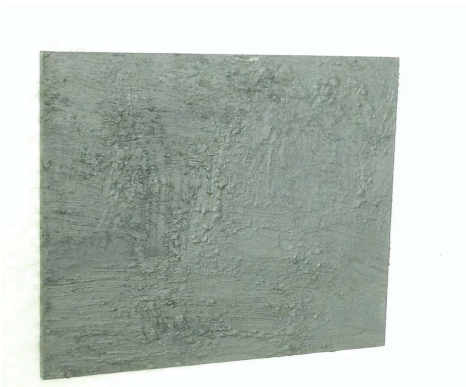
Figure 3.26. Plastic surface painted with a mixture of platinized MoS 2 and Teflon
