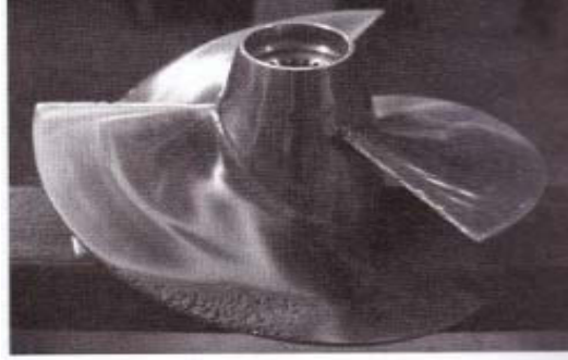
Figure 3.1 Cavitation damage to a propeller (Elger, Williams, Crowe & Roberson, 2012)
