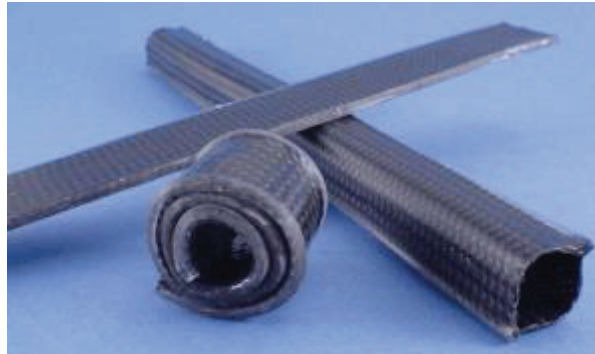
Figure 1-7. Veritex (SMP-Carbon Fiber composite). [13]
