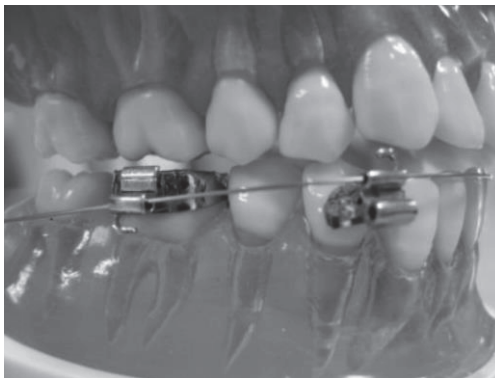
Figure 2-11. SMA orthodontic wires. [25]
