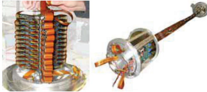
Figure 1-4. Deployable Structure Collapsed (Left) and deployed (right) [7]
