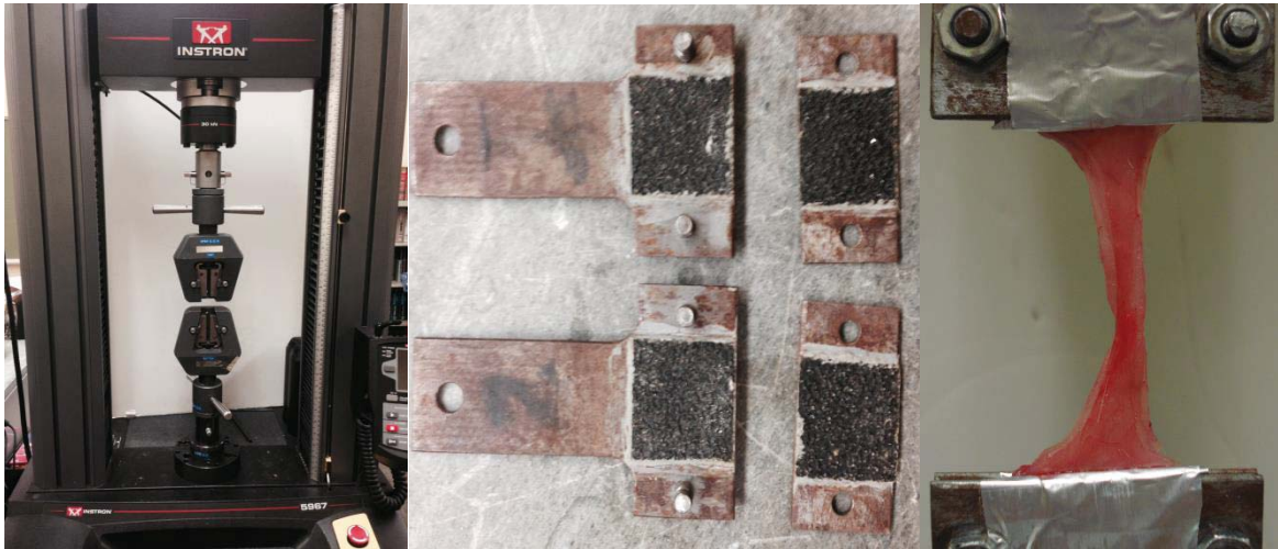
Figure 2.3: Tensile Test Equipment a) Instron Tensiometer Model 5697 equipped with 100N Load Cell b) Mechanical Grips c) Tissue Placed in Grips before Instron Test
