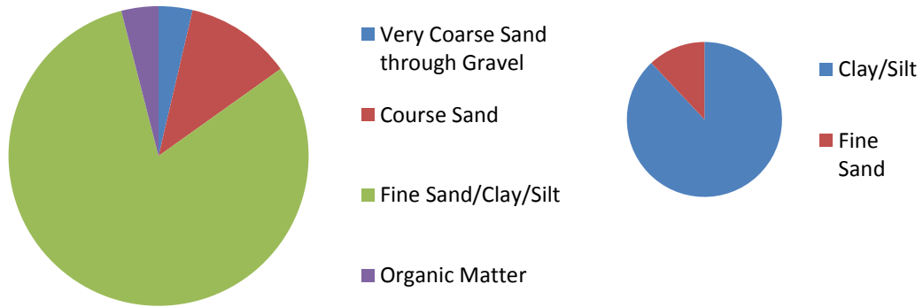
Figure 4.21 A breakdown of the Very Coarse Sand through Gravel, Coarse Sand, Fine Sand/Clay/Silt and Organic Matter for Site 2. The Fine Sand and Clay/Silt were analyzed on the Particle Size Analyzer allowing for further breakdown of the components between Clay/Silt and Fine Sand.
