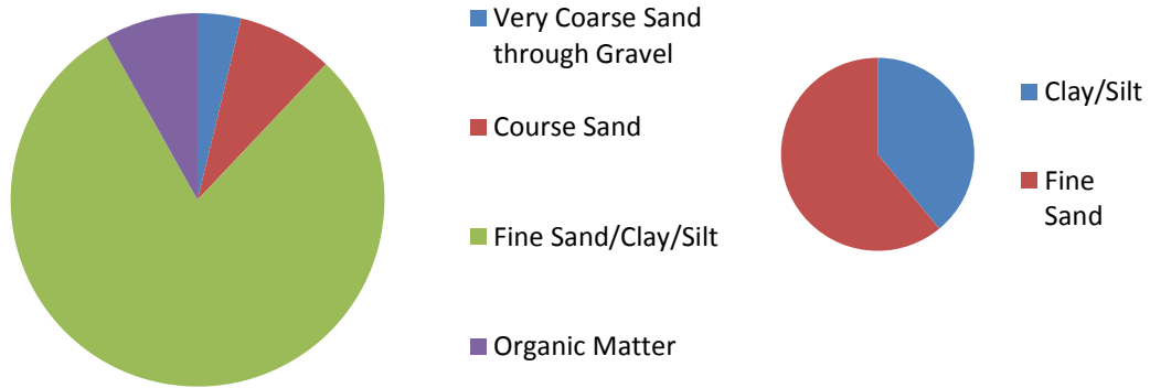
Figure 4.23 A breakdown of the Very Coarse Sand through Gravel, Course Sand, Fine Sand/Clay/Silt and Organic Matter for Site 4. The Fine Sand and Clay/Silt were analyzed on the Particle Size Analyzer allowing for further breakdown of the components between Clay/Silt and Fine Sand.
