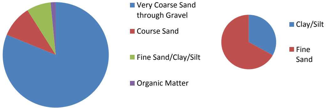
Figure 4.19 A breakdown of the Very Coarse Sand through Gravel, Coarse Sand, Fine Sand/Clay/Silt and Organic Matter for Site 0. The Fine Sand and Clay/Silt were analyzed on the Particle Size Analyzer allowing for further breakdown of the components between Clay/Silt and Fine Sand.
