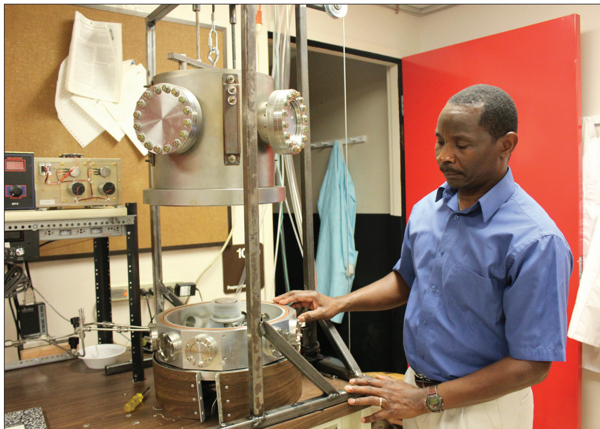
Tom Oder, professor of physics and astronomy, demonstrates the rudimentary plasma etching system that he and his students built themselves in Ward Beecher Hall.
