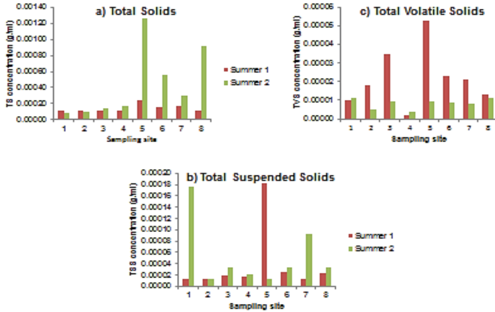
Figure 6.2 – Comparison of sedimentary data (a = TS, b = TSS, and c = TVS) from Summer 1 (shown in red) and Summer 2 (shown in green) sampling dates.
