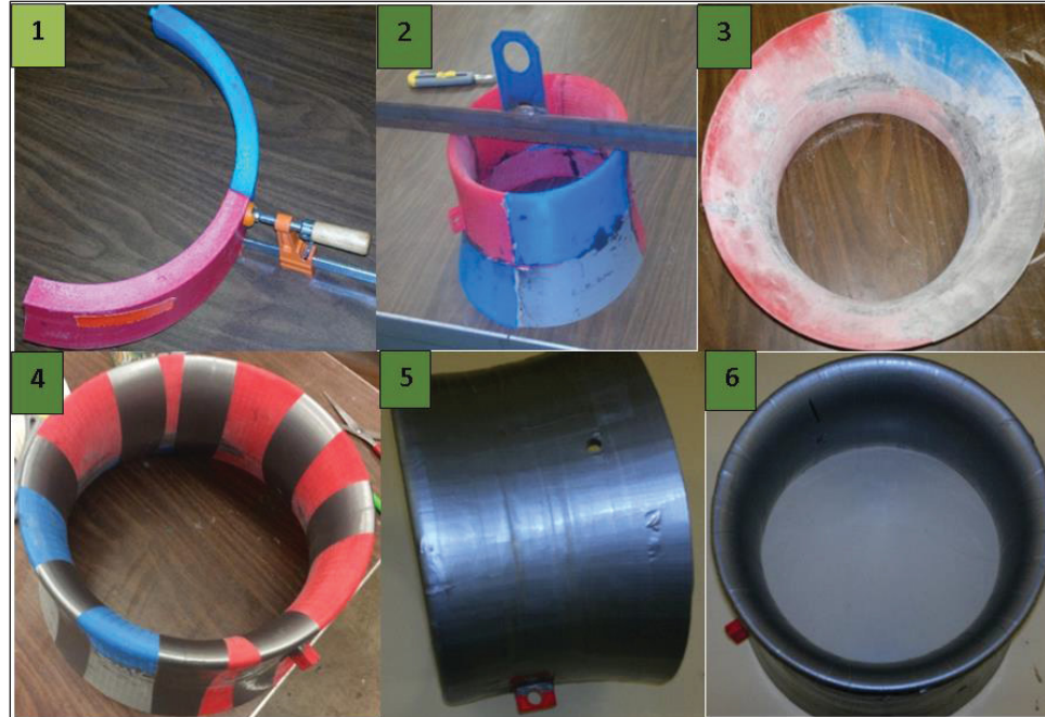
Figure 4.16 Experimental shroud (Shroud manufacturing steps): (1-2) glued parts together (3) sand the surfaces to be smooth (4) taped the whole model (5-6) complete model
