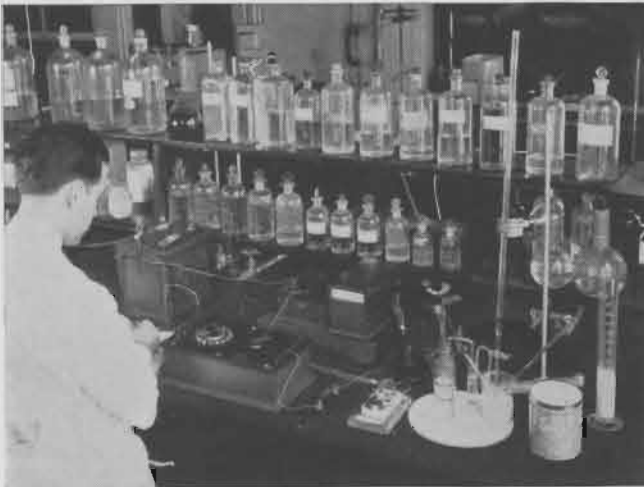
This photograph shows the equipment for determining hydrogen ion concentration necessary to plot the Buffer Curve. The chemist drops a measured quantity of acid (from the tall tube in the right foreground) into solution to be tested (in the beaker below) and records the readings from the dial before him.
