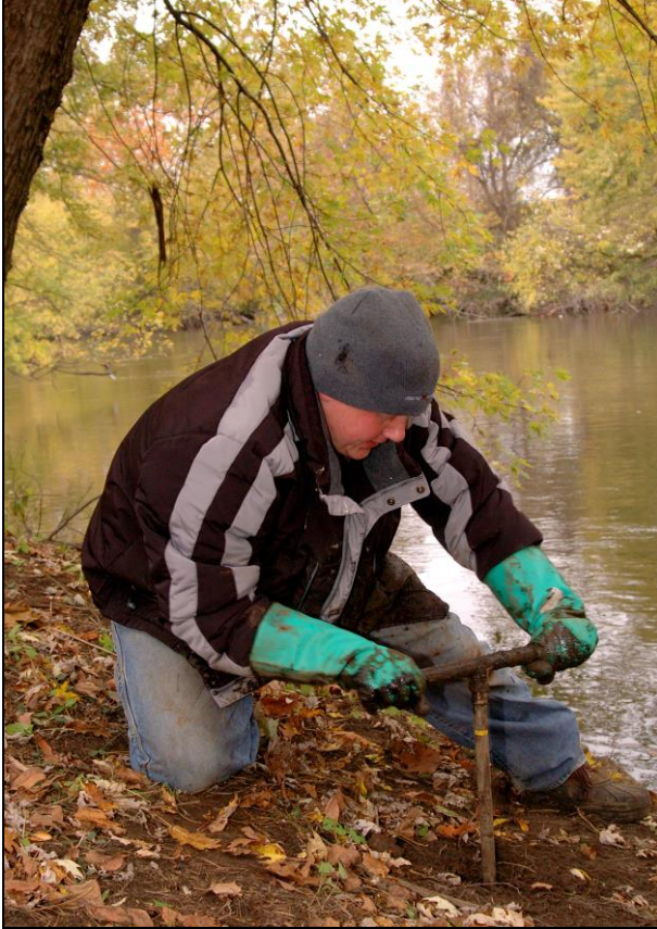
Figure 4: Hand Auger Collection of Sediment Samples
