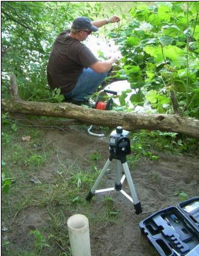
Figure 8: Gauging of River and Monitoring Well Water Elevations
