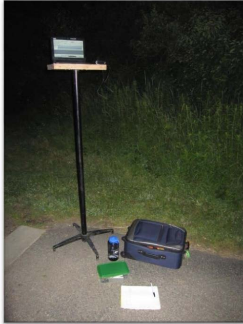
Figure 3.5 – Acoustic data collection equipment setup: ultrasonic detector and Acer netbook elevated on 1.5 m stand with a notebook and pen and equipment cases on the ground.
