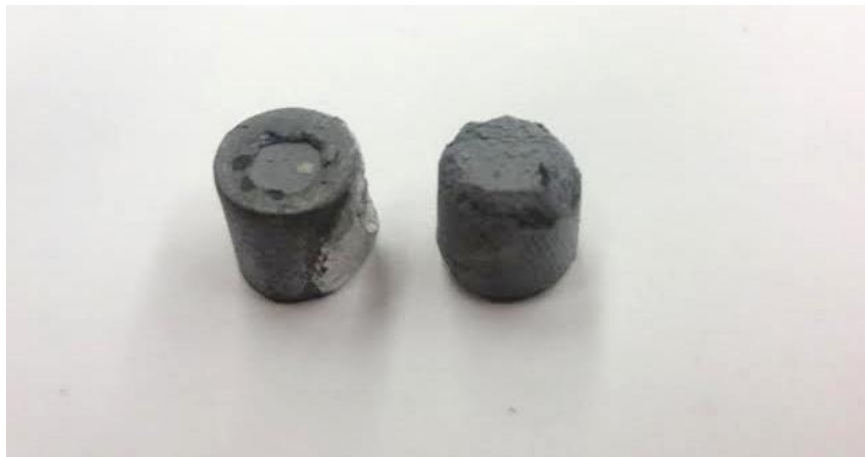
Figure 5.33. Composites samples, which were sintered at 1500°C, after split Hopkinson testing. The samples display “flaking” nature of the outer porous region.
