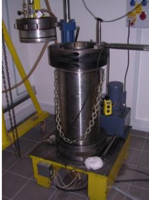
Figure 5.40. Pressure chamber used for infiltrating molten aluminum into sintered silica parts.
