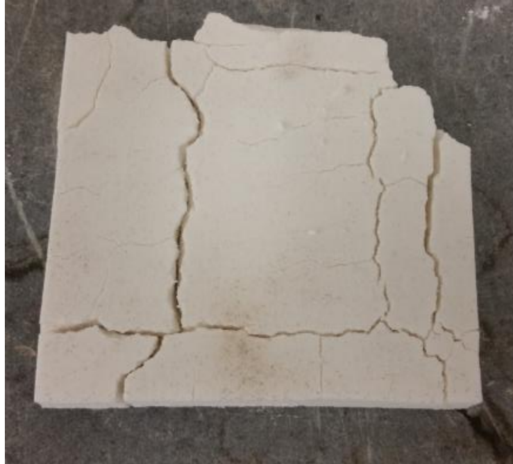
Figure 5.35. Image of a sintered 101.6 x 101.6 x 12.7 mm plate which initiated large cracks during the sintering process.
