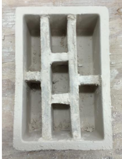
Figure 5.21. Special fixture used for a simultaneous infiltration of the 48 \mu\text{m} specimens sintered at different temperatures simultaneously.
