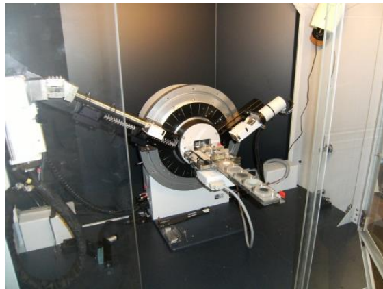
Figure 3.7. Image of the Bruker D8 diffractometer used in this research work.
