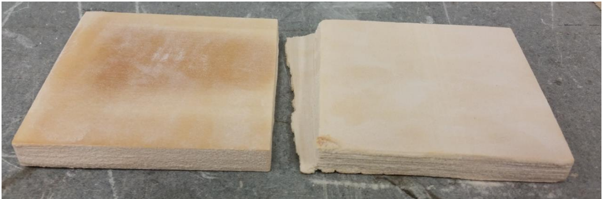
Figure 5.34. Image of the binder jetted 101.6 x 101.6 x 12.7 mm plates printed on the M-Flex.
