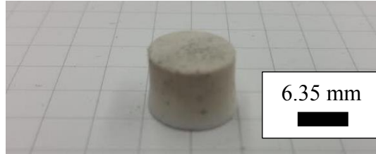
Figure 5.38. Image of the 1650°C sintered part that was designed with a 5-degree taper.
