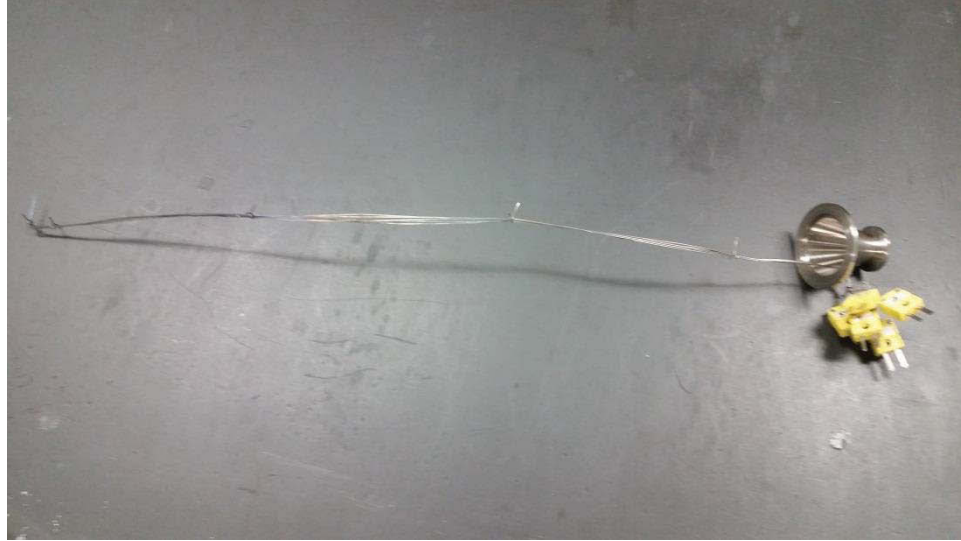
Figure 12 - Interior thermocouples and fitting
