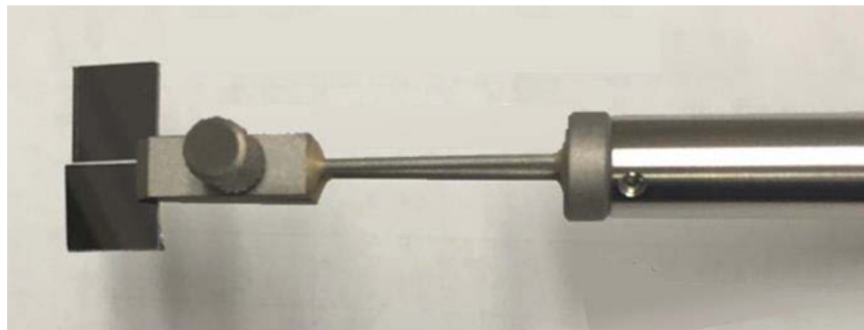
Figure 17 - Plasma cleaner sample holder with silicon substrates
